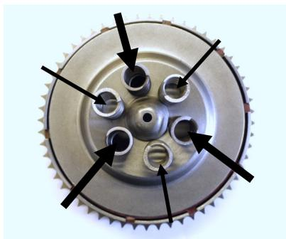
of both. This combination will give a light lever action with good 'bite' on the clutch plates. If a combination of heavy and light springs is used, fit the springs alternately: one light, one heavy spring (as in the picture on the right).
