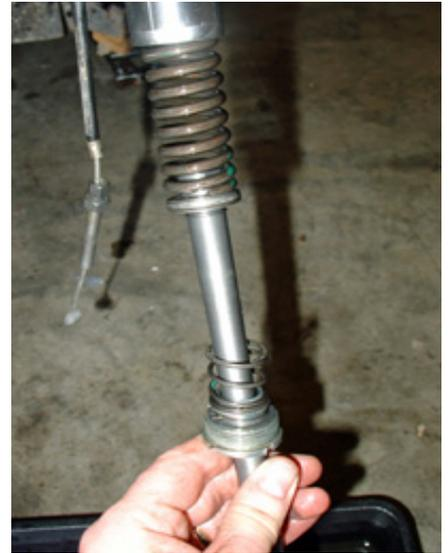
Fit the oil control collar on to the fork spring stud, with taper facing upwards. Again, a little grease will help to hold it in place on the spring stud.
