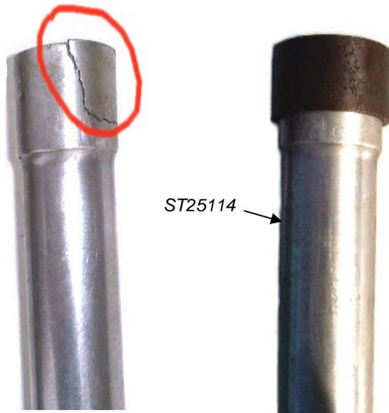
For the next step, we strongly recommend the use of the special tool, part ST25114 'Fork oil seal removal sleeve'. This tool slips over the top of the alloy fork end and prevents excess leverage cracking the alloy whilst removing the seals. With this sleeve in place, use an old tyre lever or strong screwdriver to lever out the first fork seal, then the nylon spacer and finally the second fork seal. These fork seals can be tight, heat or hot water applied locally to the fork end may help.
