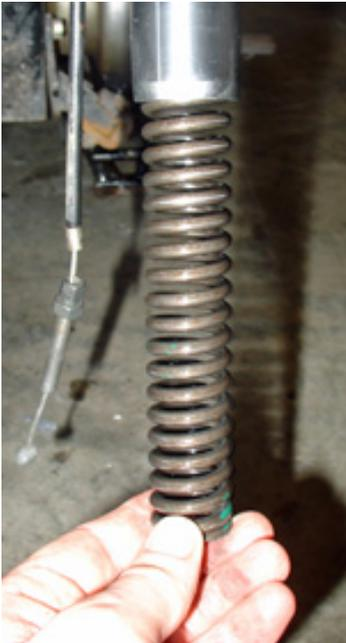
Slide the springs into the fork tubes, insert the fork spring stud with the fork valve port, tighten the valve port using the special spanner already referred to.
