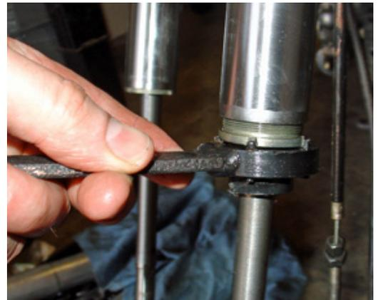
Before reassembly, clean out the fork ends, removing all the old oil. Now is a good time to check for play between the fork end and the main tube. There are no bushes fitted to this type of fork, so if the play is excessive you will need to replace the fork ends. Also make sure the main tube is not scratched or rusty, as this will damage the fork seals and create oil leaks if left unattended. Smooth out any imperfections using 1000 grade wet & dry paper with a little oil.
