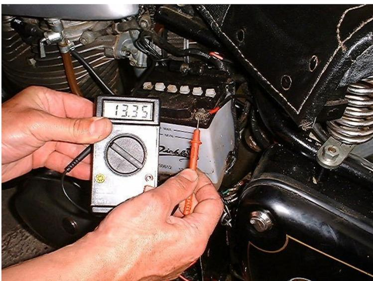
If your ammeter readings indicate a problem with the charging system then a careful examination is the only way to be certain of the fault(s). Starting at the battery, check for corroded or loose connections, electrolyte levels, fuse and earth lead security. With your multimeter set to the dc scale, check the input between the two battery connections. With the engine running this should be between 13 and 14.9 volts. (See photo on left).
