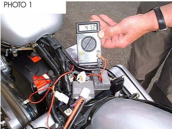
regulator / rectifier, across the black and red/yellow wire, but on the dc volts scale. This should be between 13 and 14.7 volts at the same revs. *(photo 2)*
