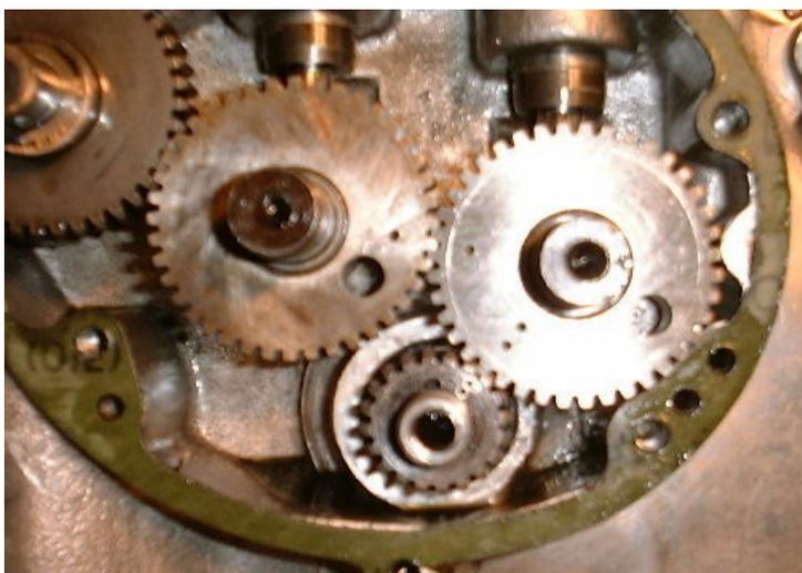
Refit the exhaust cam, lining up the 2 dots with the dots on the timing pinion.
