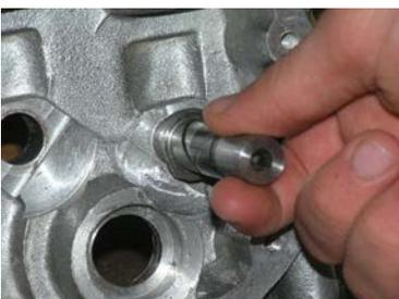
Push in the modified cam spindle and trial fit the cam. Note where the cam lobe is hitting the case. Remove the cam and spindle and grind a little where it was hitting. Repeat this step until the cam rotates freely throughout its entire 360 degrees of travel.
