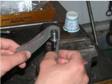
Procure a new replacement cam spindle **BEFORE** proceeding. Place one of the cam spindles in a vise and use emery cloth tape to reduce the diameter of the case end enough to where the spindle will be a tight slip fit into the case. This is so you can push it in and take it out for measuring purposes.
