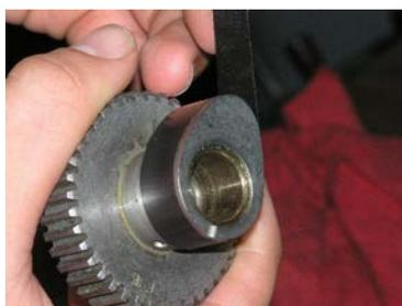
Start wrapping electrical tape around the cam. Start in the middle between the high and low points of the cam and always end a wrap there. This will insure that the same number of layers of tape exists on both ends of the cam. Put as many layers of tape on as is needed to achieve a measurement between the high and low points of the cam that is equal to the figure obtained in step 2 + .040 (+ .002/ - 0). This will give you a .020 (+ .001/ - 0) layer of tape on the high point of the cam.
