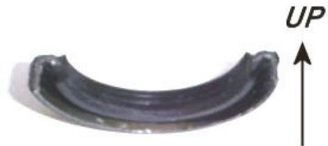
If the “oil control collar” needs to be re-fitted on the spring stud, now is the time with taper facing upwards. Again a little grease will help to hold it in place on the spring stud.
