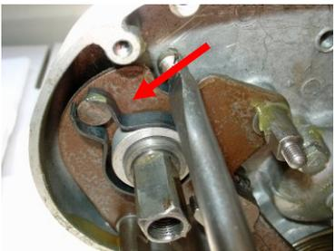
Lightly smear all the foot control ratchet components with grease to prevent corrosion and place them over the foot control shaft in the order shown in the picture on the right.
