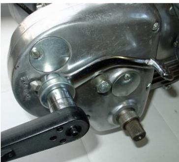
Remove the kick-start lever and gear lever. If they are tight, carefully ease the split open with a broad-bladed screwdriver. Remove the neutral finder components. Unscrew the centre bolt and remove the spring cap, spring, washer, gear indicator, neutral lever and washer. It will help in reassembly if these parts are carefully laid out in their correct order, or threaded together with wire or a nylon cable tie, as in the photograph.
