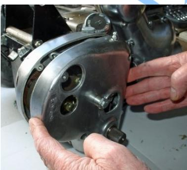
Remove the upper and lower inspection covers and disconnect the clutch cable. Note the upper cover has a longer screw, the lower cover a shorter screw.
