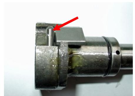
Reassembly begins with relocating the kick-start shaft in the inner case. Turn the shaft so the pawl is held 'closed' against its spring. Position the inner cover over the main gearbox case, making sure the foot operating lever locates over the arm spigot of the inner gear operator (parts arrowed in the pictures).
