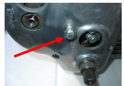
Five screws and a number of other components must be removed before the inner cover is lifted away from the gearbox. Undo the two nuts that secure the foot control stop plate and remove the washer (as arrowed in the picture). Lift the stop plate away, followed by the inner ratchet, the outer ratchet assembly and figure of 8 ratchet spring. **Do not remove the adjuster plate** behind these components or loosen the studs, as this will affect the gear selector adjustment.
