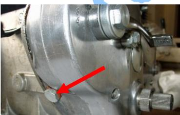
Top-up the gearbox lubricant to the correct level using the level plug located in the gearbox inner cover (arrowed in the picture). If the gearbox is packed with grease, top-up with standard 20w-50 engine oil—and the job is done!
