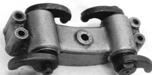
From mid-1960, the rocker housing was a one-piece alloy casting fitted with composite rockers and secured by two studs at either end, plus the centre stud for the rocker cover which screws through and helps secure it. The composite rockers, quieter in operation and much longer wearing than the earlier type, have an 11/16" diameter spindle with the arm at each end located by a flat and secured with a nut and washer.
