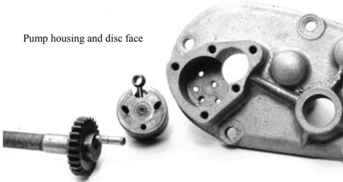
the 1957/8 models as these used the bigger feed plunger as standard. Inspect the peg closely for cracks as very occasionally they can break off, with disastrous results.
