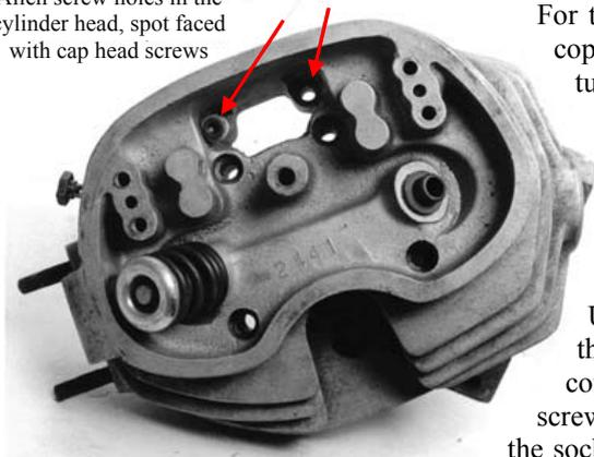
For the first two years of production the cylinder head was in cast iron with a copper/asbestos gasket to the barrel; oil leaks at the joint around the pushrod tunnel were common. In 1959, an aluminium head was used, with a boss in the pushrod tunnel and a single Allen screw helping to secure the joint.
