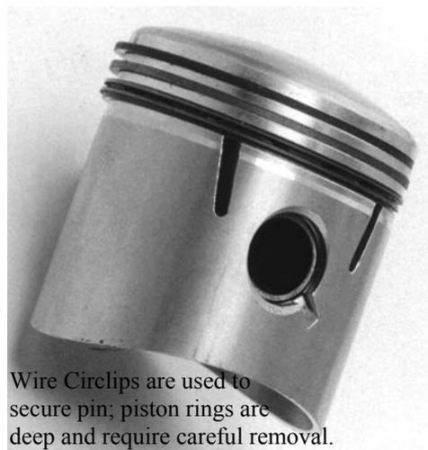
Wire Circlips are used to secure pin; piston rings are deep and require careful removal.
