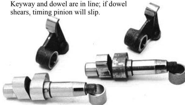
moment?), and it is therefore better to rectify the trouble straight away. Careful work with a drill is required to remove the sheared part, and a new dowel can be made from a piece of 10-gauge spoke.
